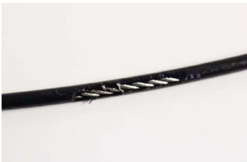
A TEAR IN THE CABLE COVER
