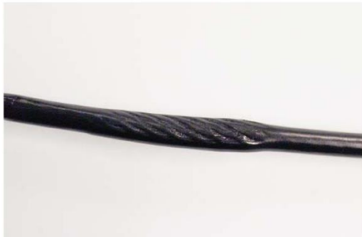
"NECKING", STRETCHED CABLE COVERING
