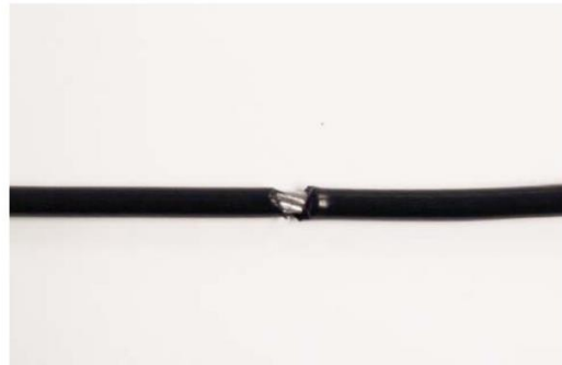
A CRACK IN THE CABLE COVER
