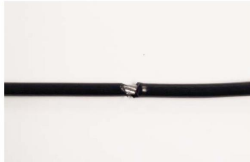
A CRACK IN THE CABLE COVER
