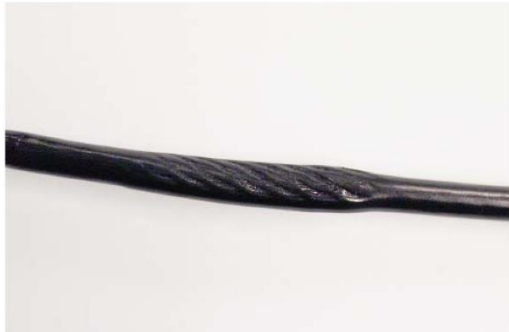
"NECKING", STRETCHED CABLE COVERING
