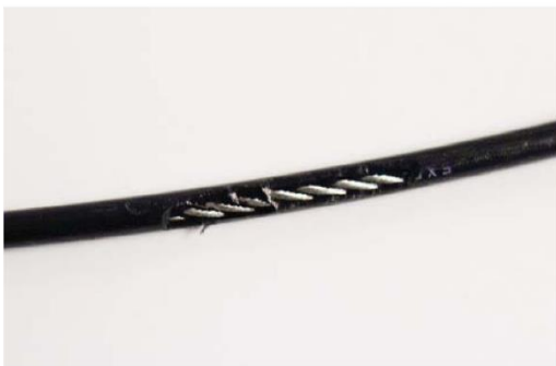
A TEAR IN THE CABLE COVER
