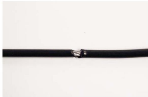
A CRACK IN THE CABLE COVER
