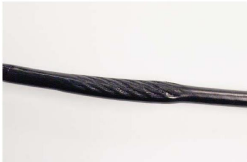
"NECKING", STRETCHED CABLE COVERING
