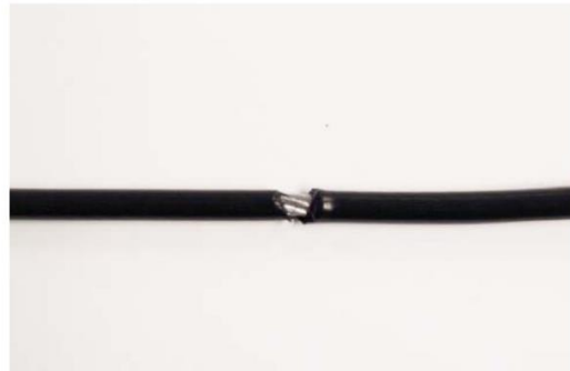
A CRACK IN THE CABLE COVER
