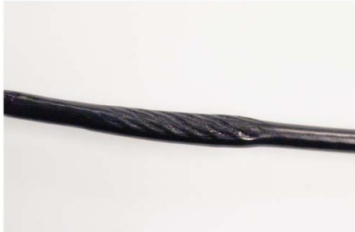
"NECKING", STRETCHED CABLE COVERING
