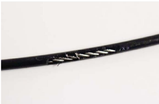
A TEAR IN THE CABLE COVER
