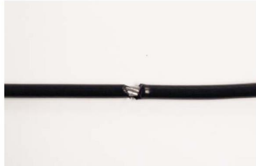
A CRACK IN THE CABLE COVER
