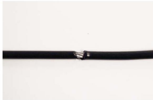
A CRACK IN THE CABLE COVER
