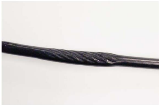
"NECKING", STRETCHED CABLE COVERING
