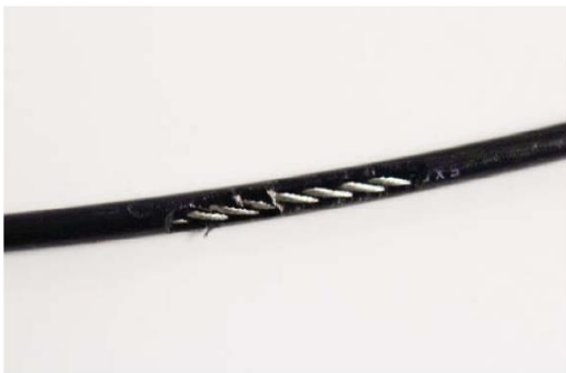
A TEAR IN THE CABLE COVER
