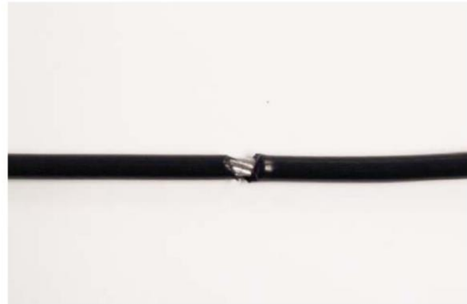
A CRACK IN THE CABLE COVER
