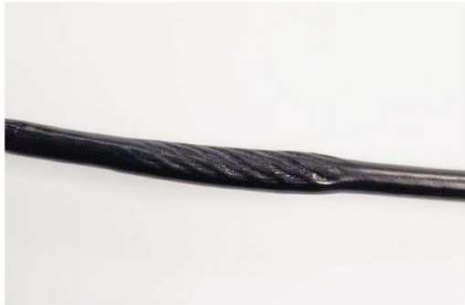
"NECKING", STRETCHED CABLE COVERING
