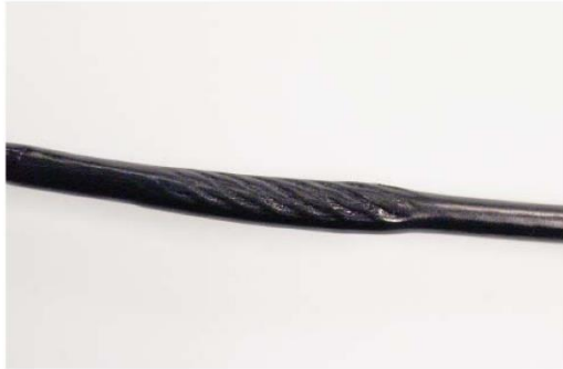
"NECKING", STRETCHED CABLE COVERING
