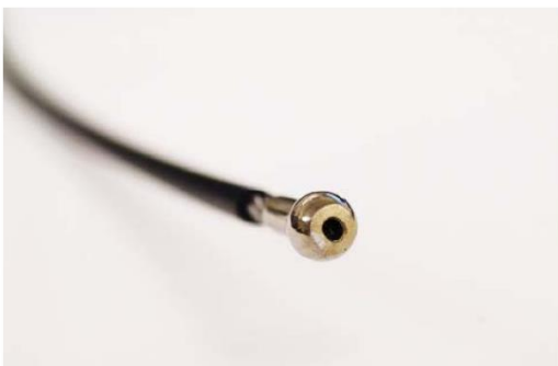
CABLE END SLIPPING OUT
