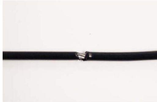
A CRACK IN THE CABLE COVER
