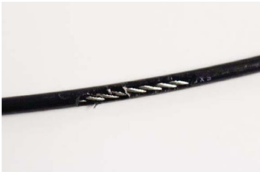
A TEAR IN THE CABLE COVER
