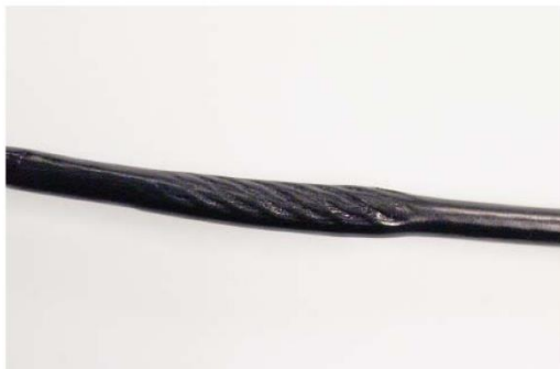
"NECKING", STRETCHED CABLE COVERING
