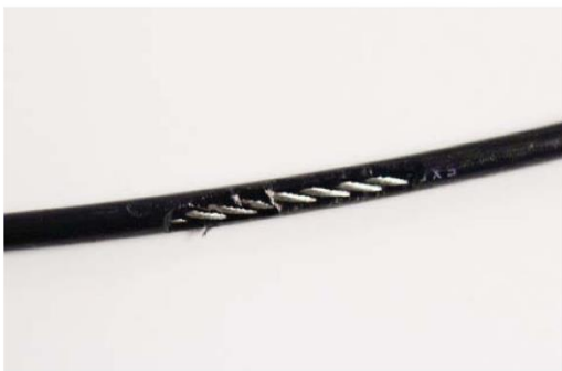
A TEAR IN THE CABLE COVER
