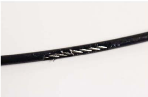
A TEAR IN THE CABLE COVER
