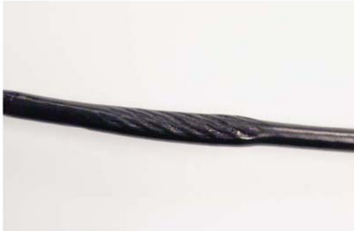
"NECKING", STRETCHED CABLE COVERING
