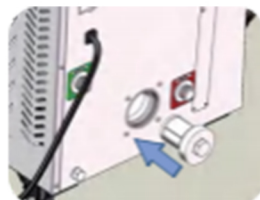
Put in the clean mesh filter.
