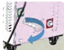
Close the lid with the plastic wrench
